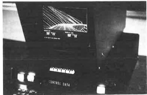
Figure 4. Highway perspective view on interactive graphics terminal.
