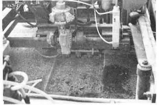
Figure 6. Smaller machine in hole-cutting operation.
