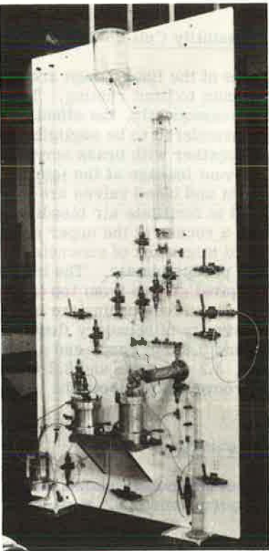
Figure 5. Permeability test equipment.
