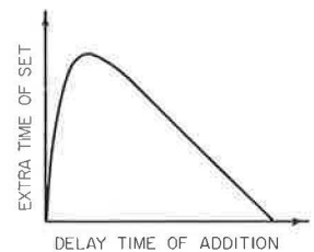
Figure 12. Extra retardation of set due to delayed addition of retarding admixture.
