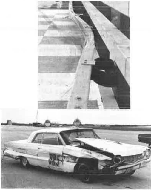
Figure 3. Condition of vehicle and collapsing-ring bridge rail after impact in test BR-5.
