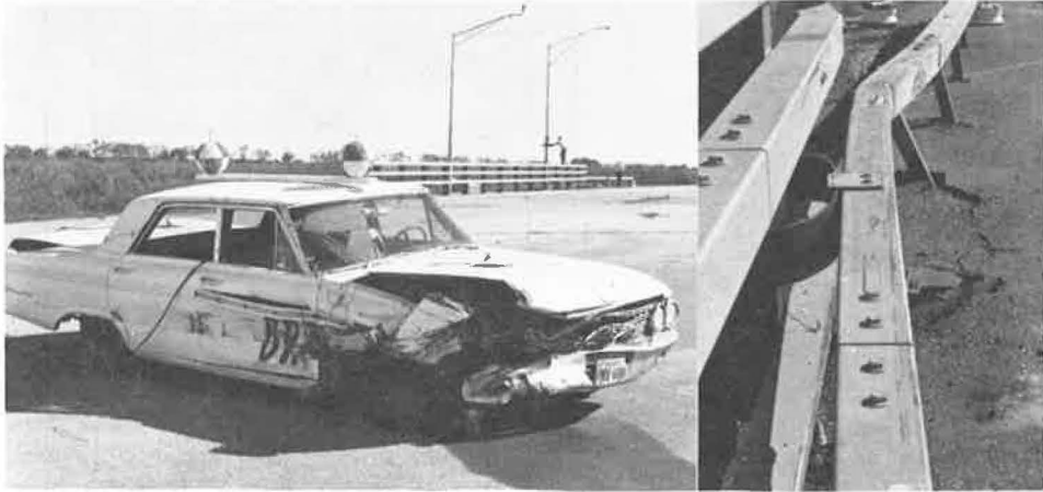
Figure 9. Condition of vehicle and collapsing-ring bridge rail after impact in test BR-7.
