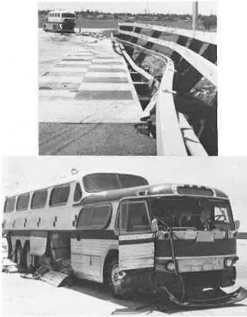
Figure 14. Condition of vehicle and collapsing-ring bridge rail after impact in test BR-9.
