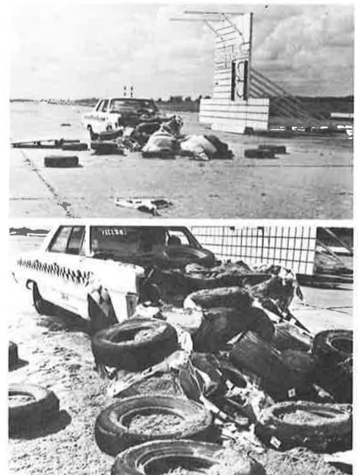
Figure 9. Test I-4 vehicle and barrier after impact.
