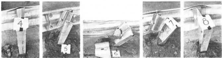
Figure 7. Barrier damage, test 276.
