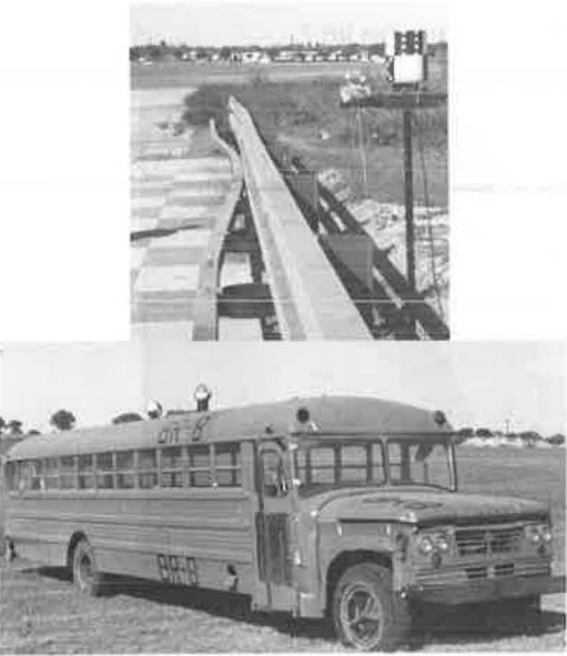
Figure 11. Condition of vehicle and collapsing-ring bridge rail after impact in test BR-8.
