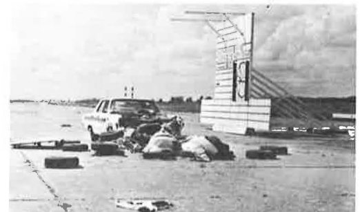
Figure 9. Test I-4 vehicle and barrier after impact.
