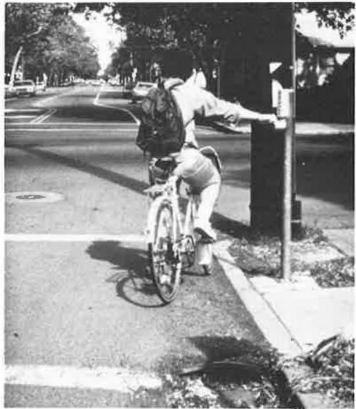
Figure 21. Push-button signal for bicyclists that activates traffic signal.
