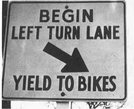
Figure 19. Explicit sign warning motorists of bicycle's presence in Seattle.
