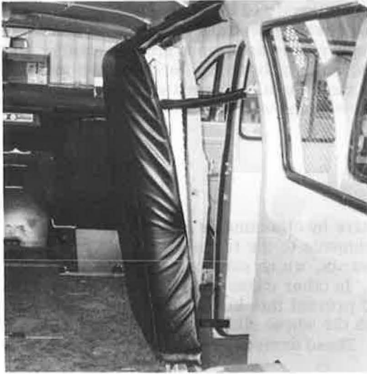
Figure 4. Inside storage of ramp with padding.
