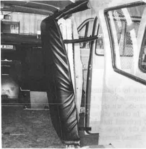
Figure 4. Inside storage of ramp with padding.
