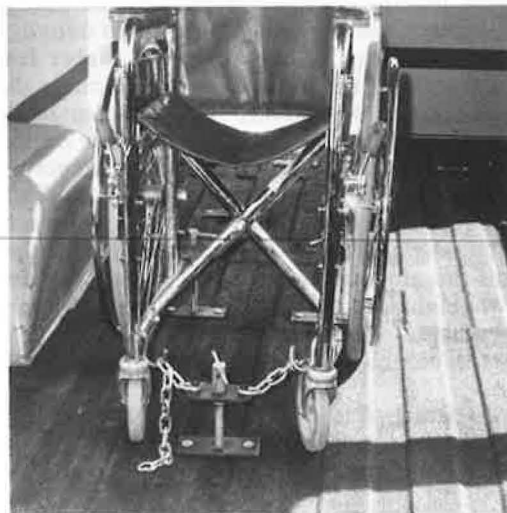
Figure 7. Chain and S-hook chair securement.
