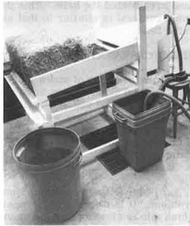
Figure 1. Apparatus for testing the trapping efficiency of a bale.
