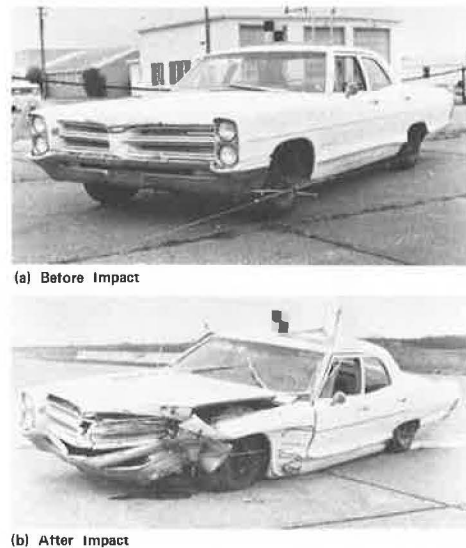
Figure 4. Test vehicle before and after impact.
