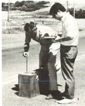
Figure 2. Impulse index computer in operation on Wash-270.
