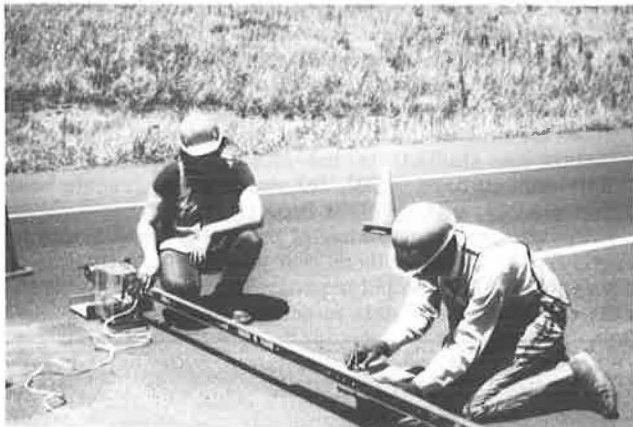
Figure 1. Transverse profile gauge.
