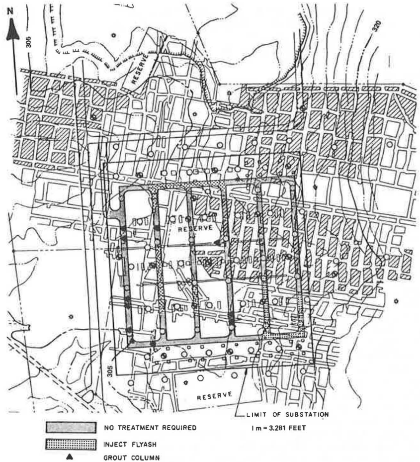
Figure 6. Roadway stabilization treatment areas in the substation.
