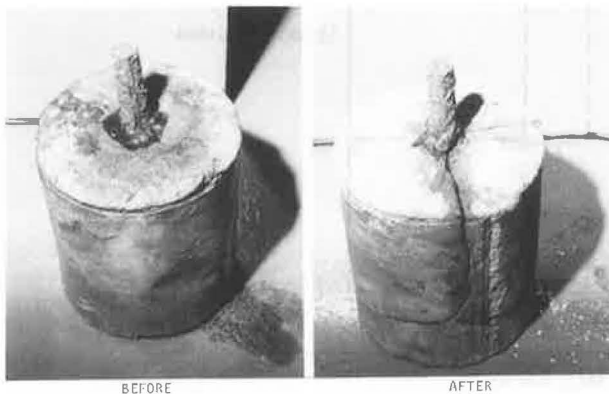
Figure 6. Before-and-after failure photographs of typical specimen.
