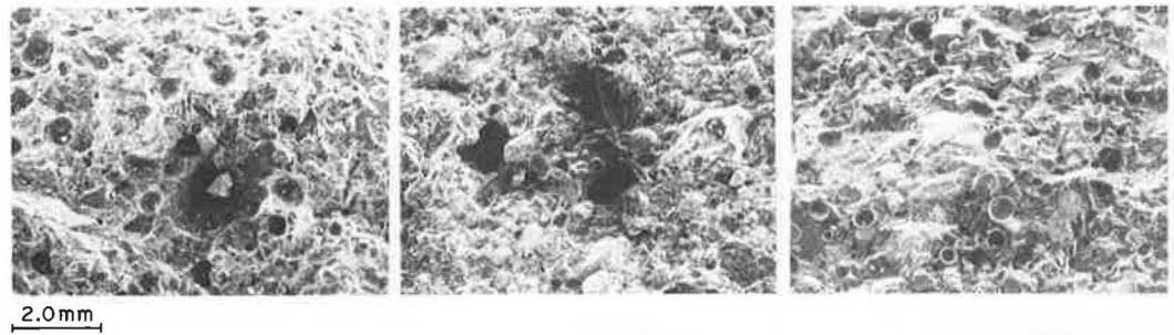
Figure 4. Scanning electron micrographs of fracture surfaces of tensile-splitting specimens of series E epoxy-cement mortars (left, E1 series with no epoxy; middle, E3 series with 40 percent epoxy replacement; right, E6 series with 100 percent epoxy replacement).
