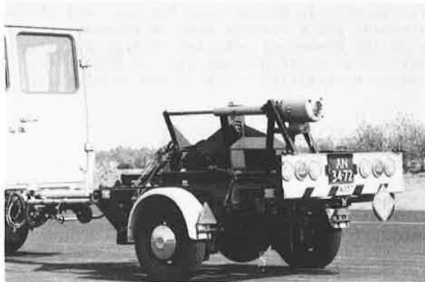
Figure 1. Skidding resistance measuring truck of the Dutch State Road Laboratory.
