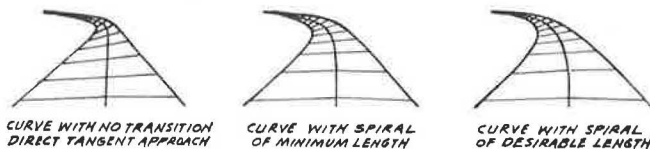
Figure 6. Perspective of roads with spiral curves.
