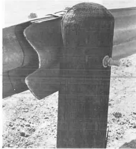
Figure 18. Post 1 with backup plate and metal clips before test 3.
