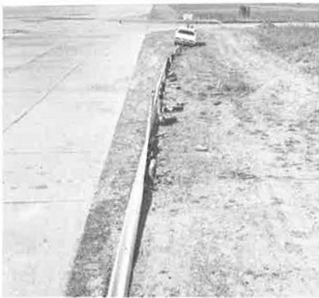
Figure 24. Position of vehicle and damage to guardrail and terminal after test 5.
