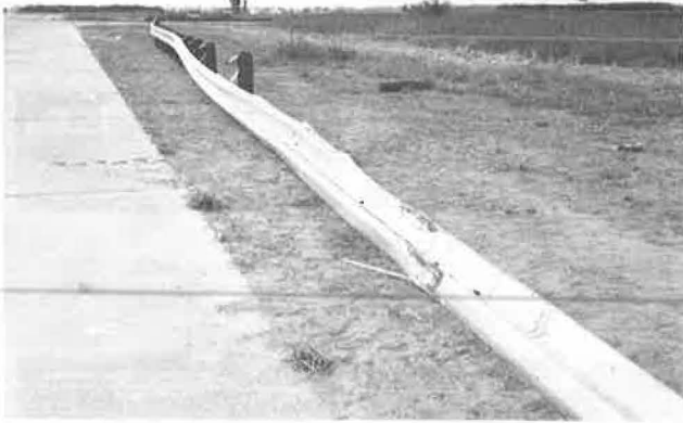
Figure 14. Guardrail and terminal after test 1.
