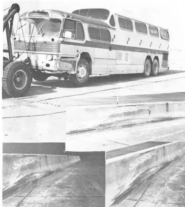
Figure 5. Damage after test CMB-22.
