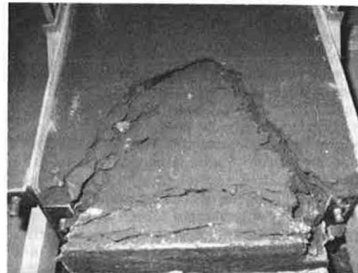
Figure 10. Cone-shaped failure in specimen with bar-mesh reinforcement.
