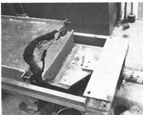
Figure 13. Cone-shaped failure in specimen with solid steel-plate reinforcement for test 7.
