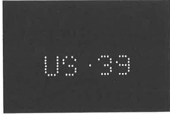
Figure 10. Route numeral at 50 percent bulb failure.
