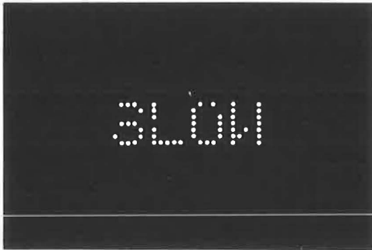
Figure 1. Four-character word at 10 percent bulb failure.
