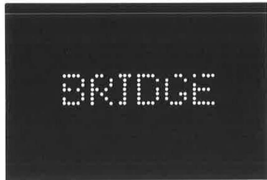
Figure 3. Six-character word at 10 percent bulb failure.
