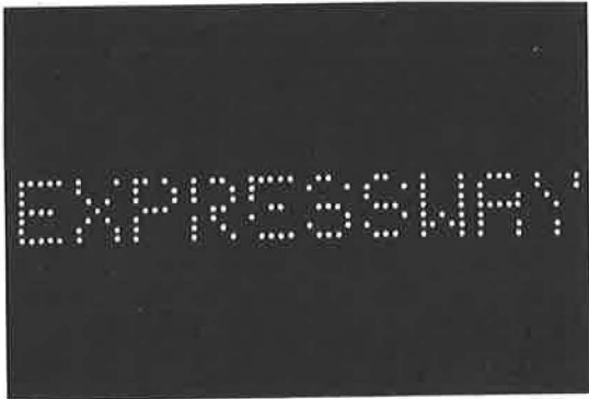
Figure 7. Ten-character word at 10 percent bulb failure.
