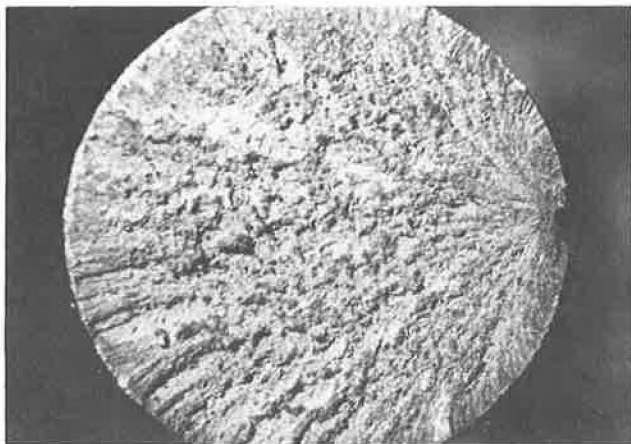
Figure 14. Typical brittle fracture of Macalloy bar.
