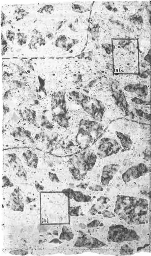
Figure 8. Slice through full thickness of core showing zones of different air content: (a) 12 percent and (b) 3 percent.
