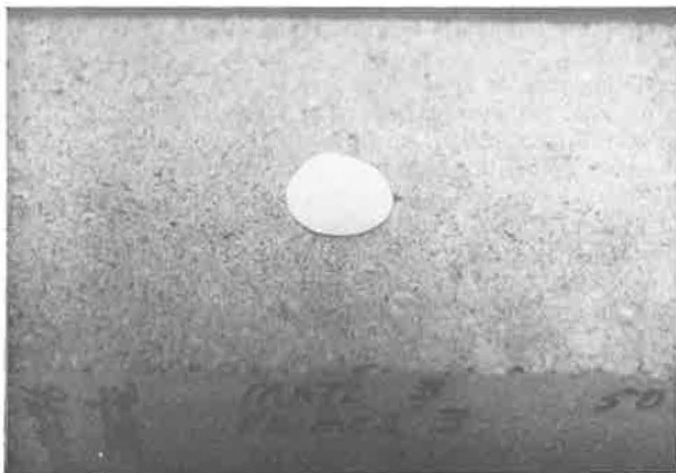
Figure 6. Teflon disk on concrete slab.
