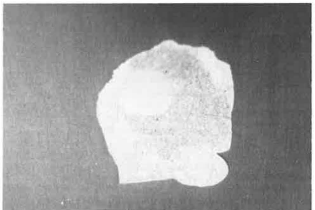
Figure 10. Previously bonded surface of thermoplastic.
