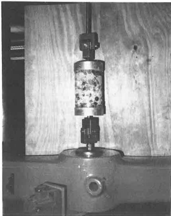
Figure 10. Apparatus for testing direct tensile bond.
