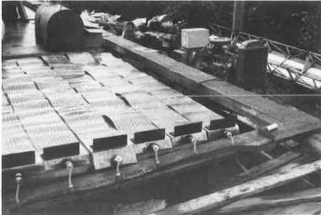
Figure 11. Electric blankets on test slab 4.
