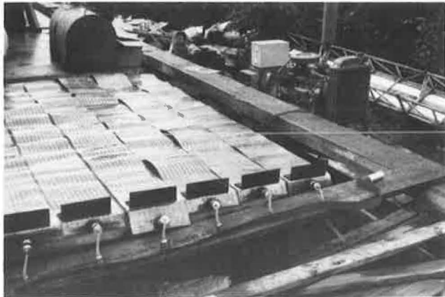
Figure 11. Electric blankets on test slab 4.
