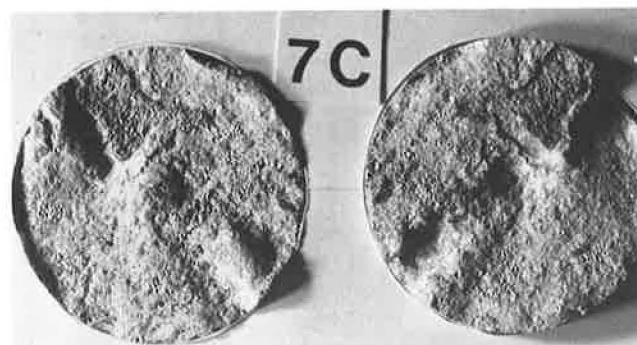
Figure 11. Results of uniaxial tensile strength tests: rupture running across whole mortar course [ \beta_z = 1.08 MPa (157 lbf/in 2 )].
