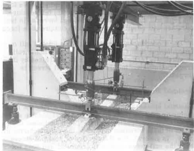
Figure 15. Laboratory tests on tie supported on ballast and subgrade.
