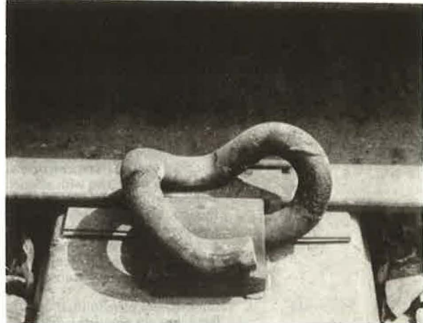
Figure 6. Rail fastener on concrete tie.
