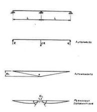
local web yielding. Although the ASD method may consider automoments to meet the Overload performance requirements, the bridge may never experience automoments unless the loading is sufficiently heavy; such behavior is acceptable.
