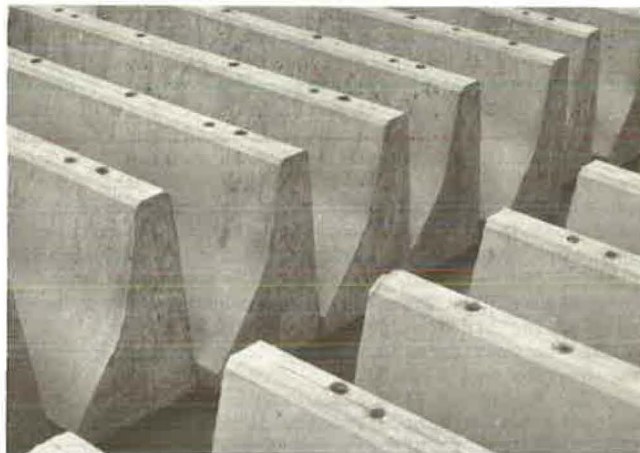
Figure 8. Modular precast parapets.
