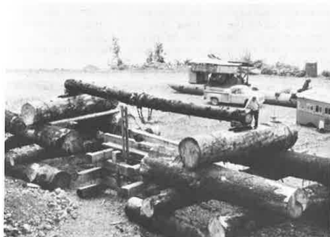
Figure 3. Test set-up (with log in position) for bending tests.
