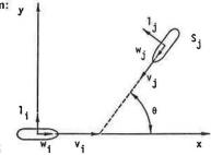
Figure 2. Collision problem: equivalent one-body system.
