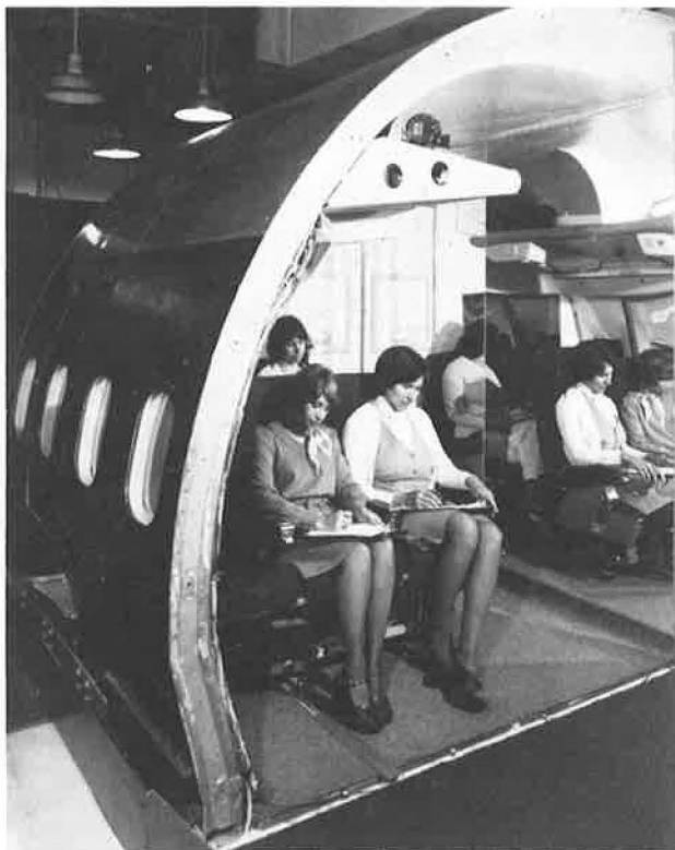
Figure 1. A view of Passenger Ride Quality Apparatus (PRQA), a laboratory simulator located at Langley Research Center, Hampton, Virginia.
