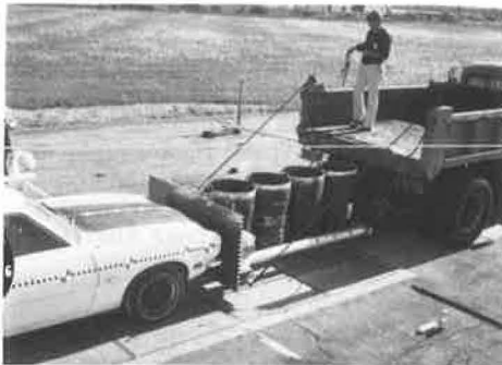
Figure 1. Two views of the portable energy-absorbing system.
