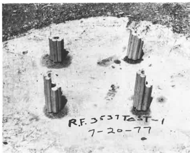
Figure 6. Closeup of coupling after breakaway.
