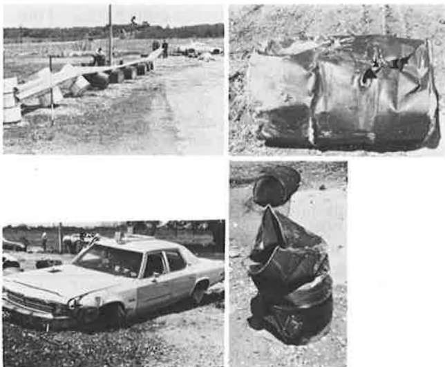
Figure 11. Test TB-5 vehicle and barrier damage.
