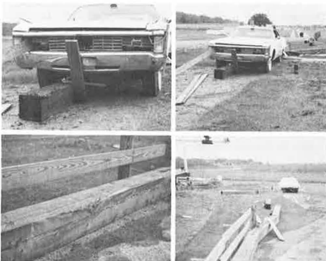
Figure 3. Test TB-1 vehicle and barrier damage.
