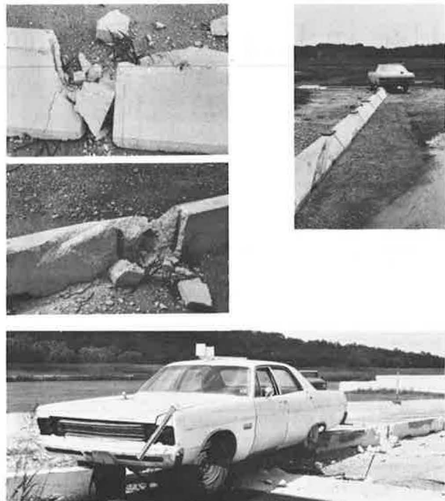
Figure 13. Test TB-6 vehicle and barrier damage.
