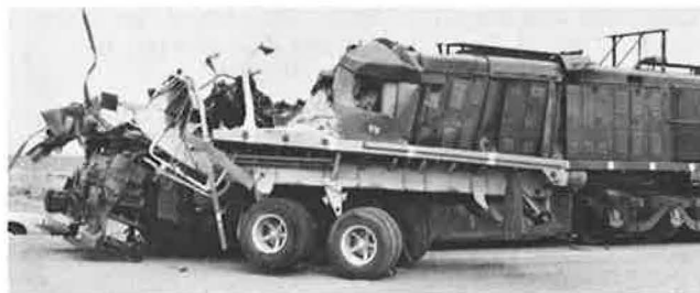
Figure 21. Frame buckling damage—full-scale grade-crossing test.
