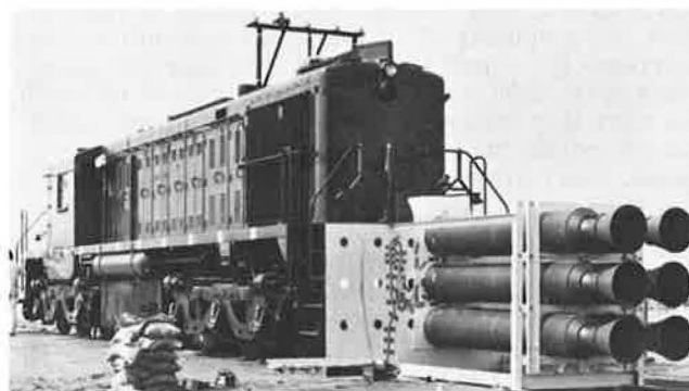
Figure 19. Rocket-powered locomotive—full-scale grade-crossing test.
