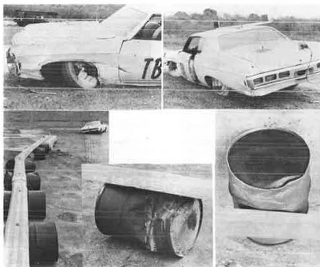
Figure 9. Test TB-4 vehicle and barrier damage.
