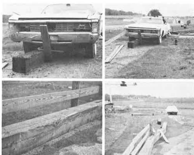
Figure 3. Test TB-1 vehicle and barrier damage.
