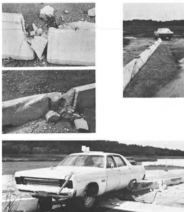
Figure 13. Test TB-6 vehicle and barrier damage.
