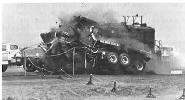
Figure 20. Full-scale impact—full-scale grade-crossing test.
