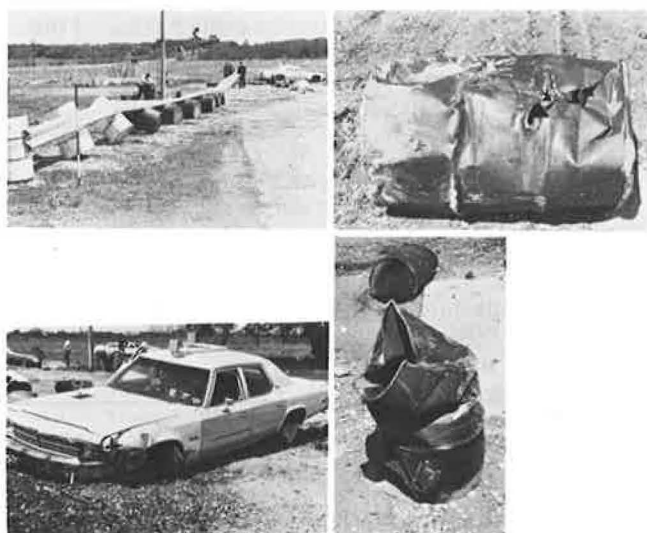
Figure 11. Test TB-5 vehicle and barrier damage.
