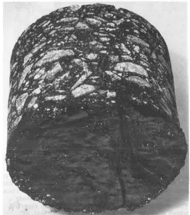
Figure 5. Core through bituminous layers and nylon fabric: I-95 project.
