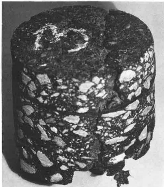
Figure 3. Core through new overlay (top), polypropylene fabric, and old overlay.
