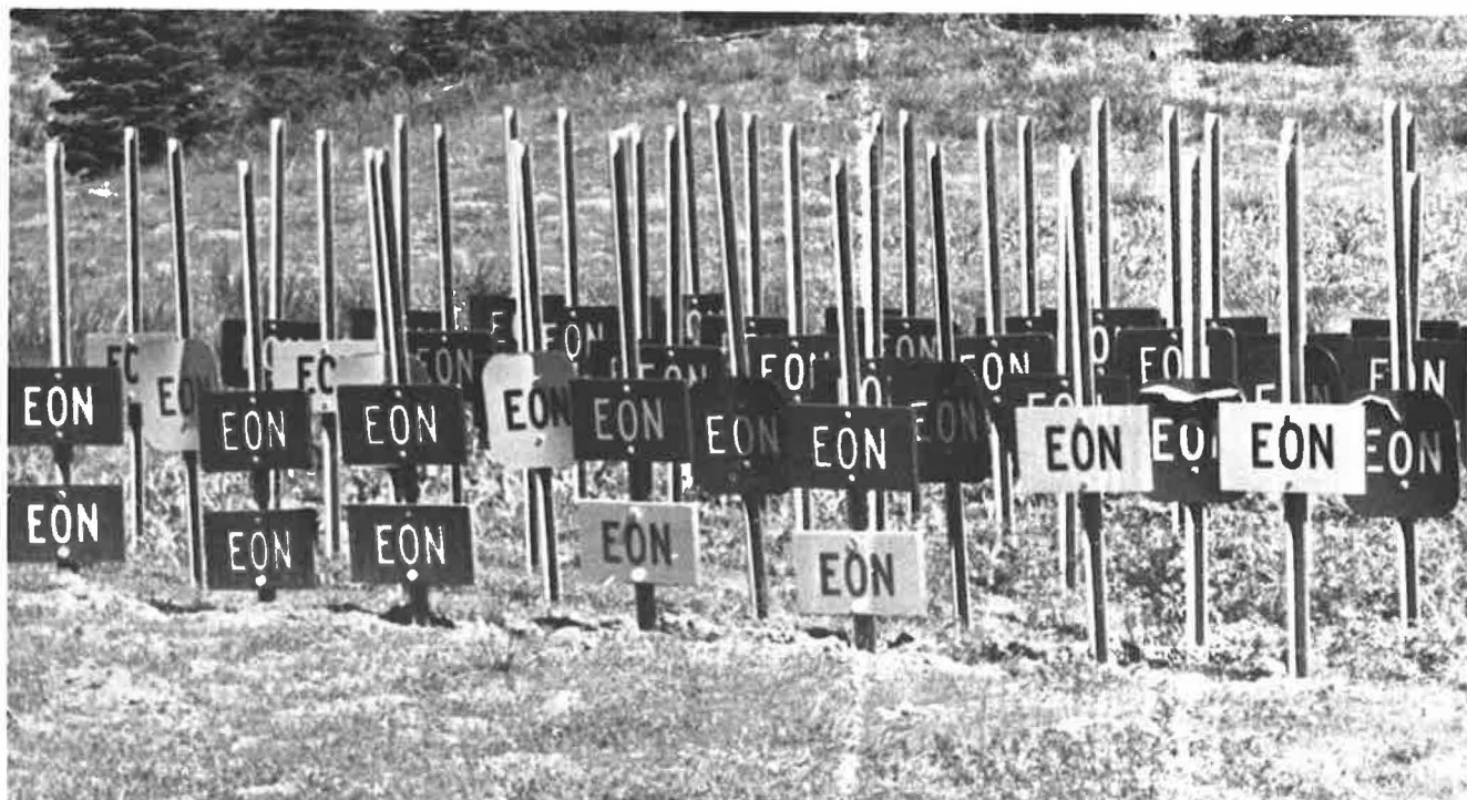
Figure 10. Signs of Mitsubishi/Seibu International materials after 2 years of outdoor exposure.
