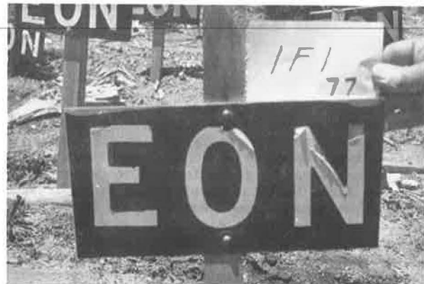
Figure 2. Test sign message is legible but maintenance would be required for esthetic purposes and to prevent further deterioration.
