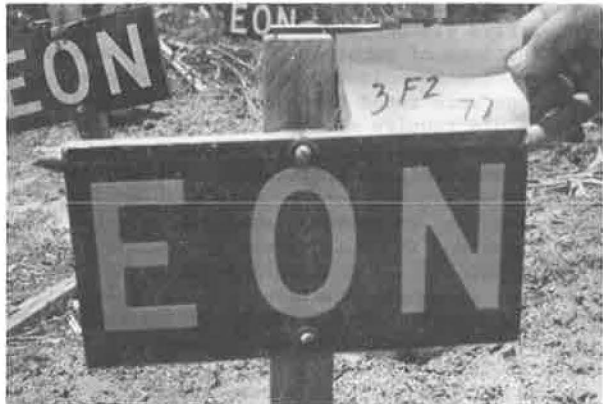
Figure 1. Test sign shows no structural failure that would require maintenance.
