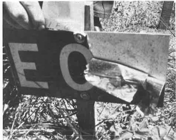
Figure 7. Background sheeting generally peeled more severely from aluminum than plywood.
