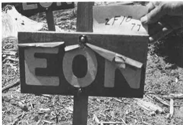
Figure 3. Test sign message is becoming unreadable and sign requires immediate replacement or repair.
