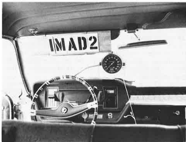
Figure 5. Vehicle interior showing taped steering wheel and large speedometer.
