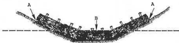
Figure 4. Proper straw barrier placement; points A should be higher than point B.
