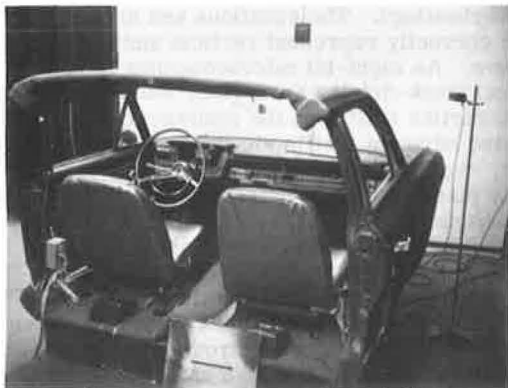
Figure 6. Automobile cab and screen with peripheral light assembly (at right) and spotlight (at top).
