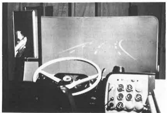
Figure 5. Video-projected truck-driving display with horizontal and vertical curvature.
