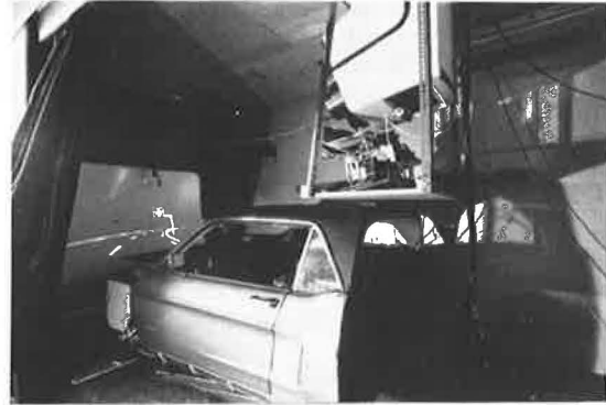
Figure 4. Projected video road image combined with slide-projected signs.
