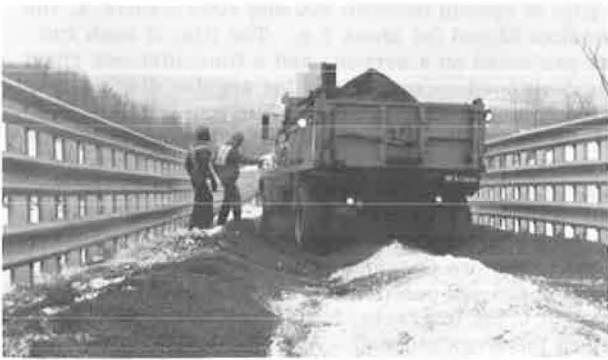
Figure 6. Final position of truck after run at 90 km/h (56 miles/h).
