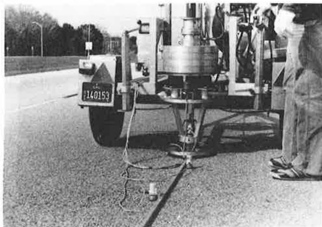
Figure 1. Falling-weight deflectometer (FWD) on I-75 near Gainesville, Florida.
