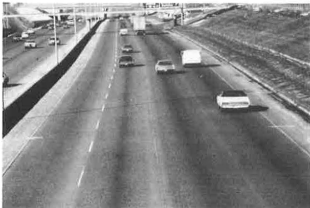
Figure 2. Condition of best-formulation epoxy (HA-1) after three years (left stripe).
