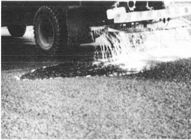
Figure 3. Infiltration test on binder course surface.
