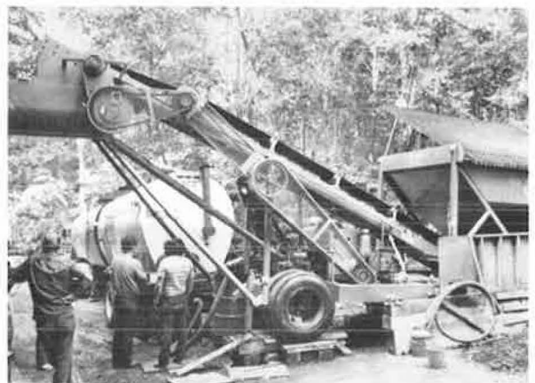
Figure 14. Portable pugmill mixing emulsion with recycle-aggregate blend.
