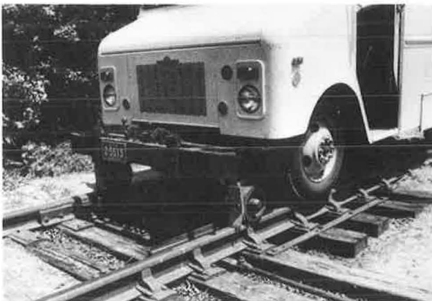
Fig. 2B Close-up of high-rail assembly engaged on track.
