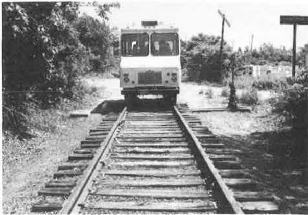
Fig. 2A Front view of rail photolog van, Chevrolet Chassis, High-rail equipped.
