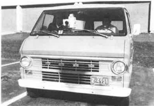
Fig. 1A Photolog Van with Camera mounted in filming position.
