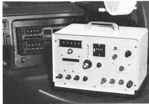
Fig. 1D Distance Measuring Instrument (DMI) and Distance Event Marker (DEM) mounted in dash.
