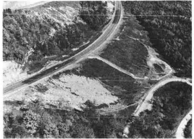
Figure 4. The Rockwood fill slide between stations 2001+00 and 2018+00 (paved areas delineate lateral limits of slide).
