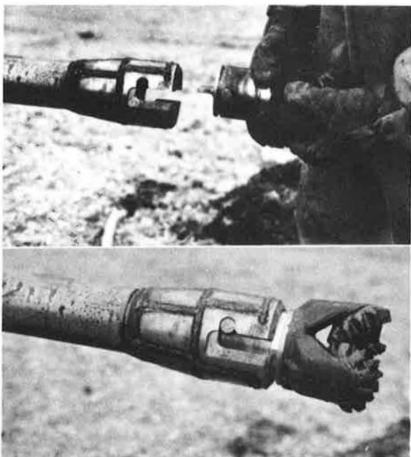
Figure 6. J-slot bit adaptor (top) and dropoff bit (bottom).
