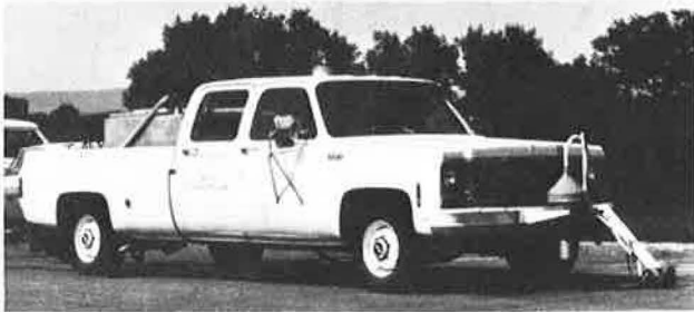
Figure 1. Skid tester and dust-collection system.
